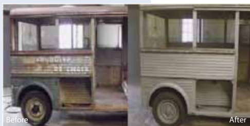
Derusting and paint removal
