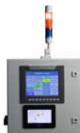
Pelletiser, scale and CO 2 detector can be controlled by a remote controller
